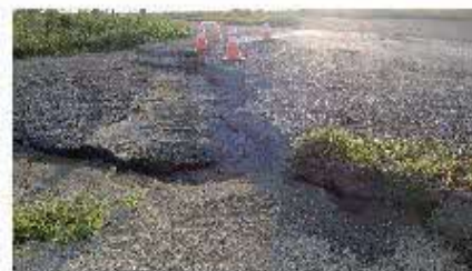
第7図 海岸低地に生じた噴砂(むかわ町美幸)。 Fig. 7 Liquefied sand boil around the lowland at the coastal area (Miyuki, Mukawa Town).
