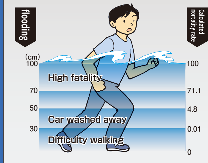
Fatalities due to tsunami and flooding
